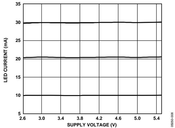
Figure 7.  $I_{LED}$  (mA) vs. Supply Voltage (V)
