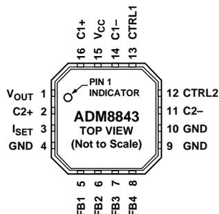
Figure 2. Pin Configuration
