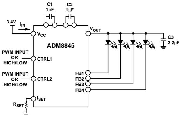
Figure 19. Digital PWM Brightness Control Application Diagram
