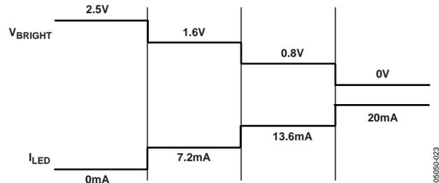
Figure 22. PWM Brightness Control Application Diagram Using a DC Voltage Applied to V<sub>BRIGHT</sub>
