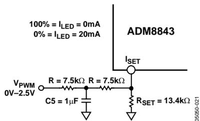
Figure 21. PWM Brightness Control Using Filter-PWM Signal
