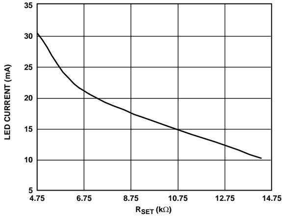
Figure 3.  $I_{LED}$  (mA) vs.  $R_{SET}$
