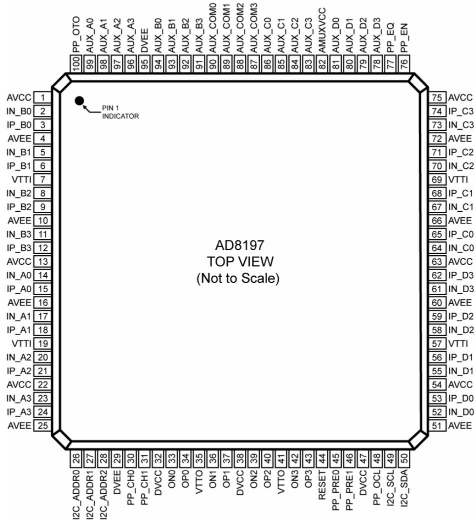
Figure 3. Pin Configuration
