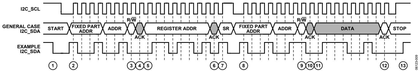
Figure 30. I<sup>2</sup>C Read Diagram
