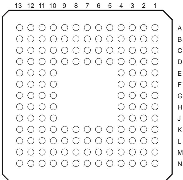
The pin assignments table to follow lists each signal quadrant and BGA ball number for the TMS320VC5402GGU (144-pin BGA) package which is footprint-compatible with the 'LC548 and 'LC/VC549 devices.
