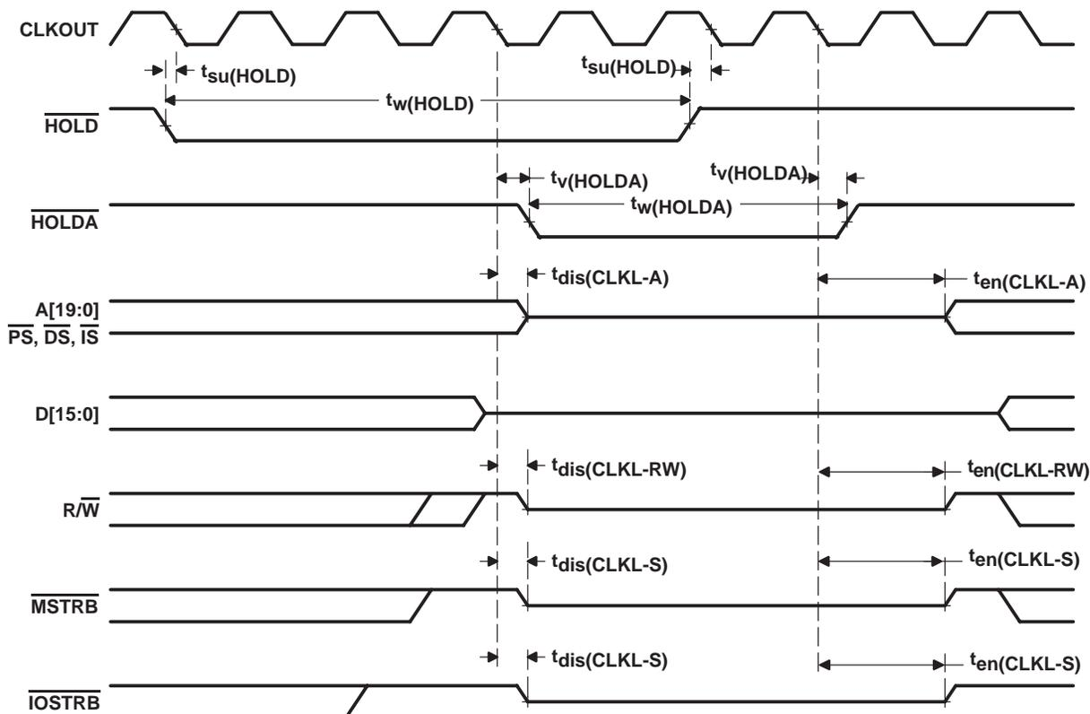
Figure 21.  $\overline{\text{HOLD}}$  and  $\overline{\text{HOLDA}}$  Timings (HM = 1)
