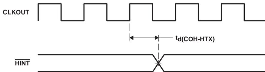
Figure 37.  $\overline{\text{HINT}}$  Timing
