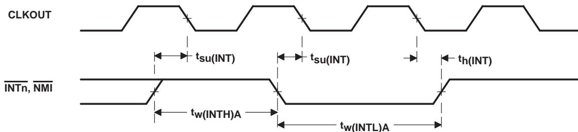
Figure 23. Interrupt Timing
