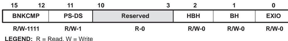
**Figure 6. Bank-Switching Control Register (BSCR), MMR Address 0029h**
