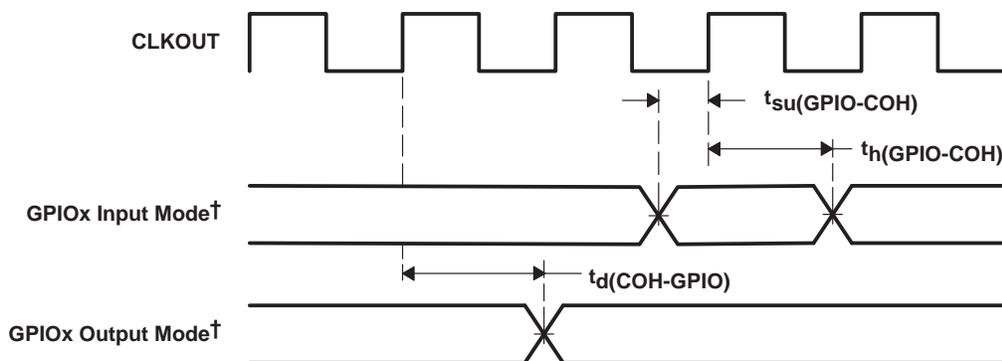
† GPIOx refers to HD0, HD1, HD2, ...HD7, when the HD bus is configured for general-purpose input/output (I/O).
