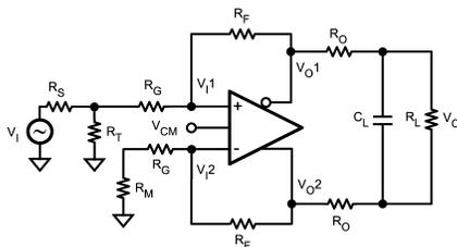
$$*V_{CM} = \frac{V_{O1} + V_{O2}}{2} \quad *BY\ DESIGN$$
