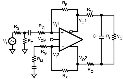
$$*V_{CM} = \frac{V_{O1} + V_{O2}}{2} \quad *BY\ DESIGN$$
