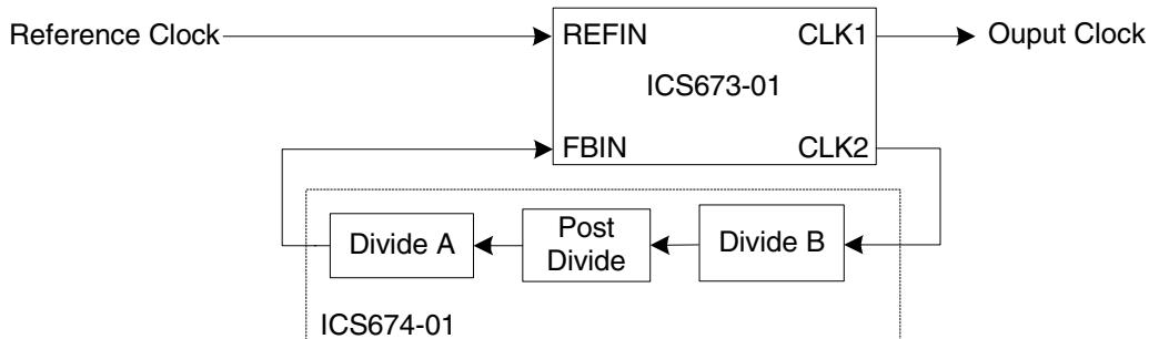
Note that in both examples, Divide B is connected to the output of the ICS673. This is because Divide B has a higher operating frequency than Divide A.
