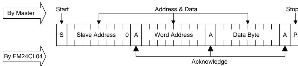
Figure 5. Byte Write
