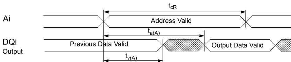
Read Cycle 2:  $\bar{G}$ -,  $\bar{E}$ -controlled (during Read Cycle:  $\bar{W} = V_{IH}$ )
