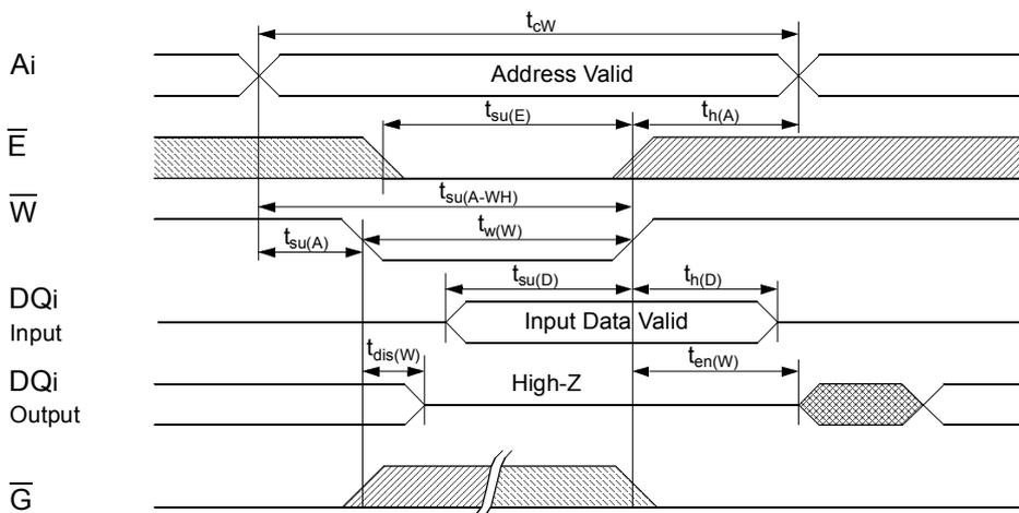
Write Cycle 2:  $\overline{E}$ -controlled
