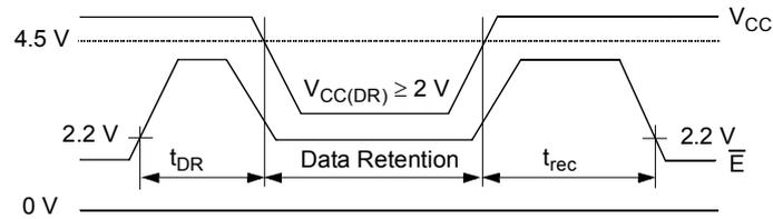
$$V_{CC(DR)} - 0.2 \text{ V} \leq V_{\bar{E}(DR)} \leq V_{CC(DR)} + 0.3 \text{ V}$$
