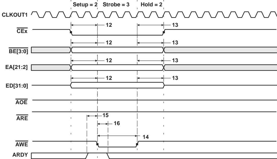
Figure 15. Asynchronous Memory Write Timing (ARDY Not Used)
