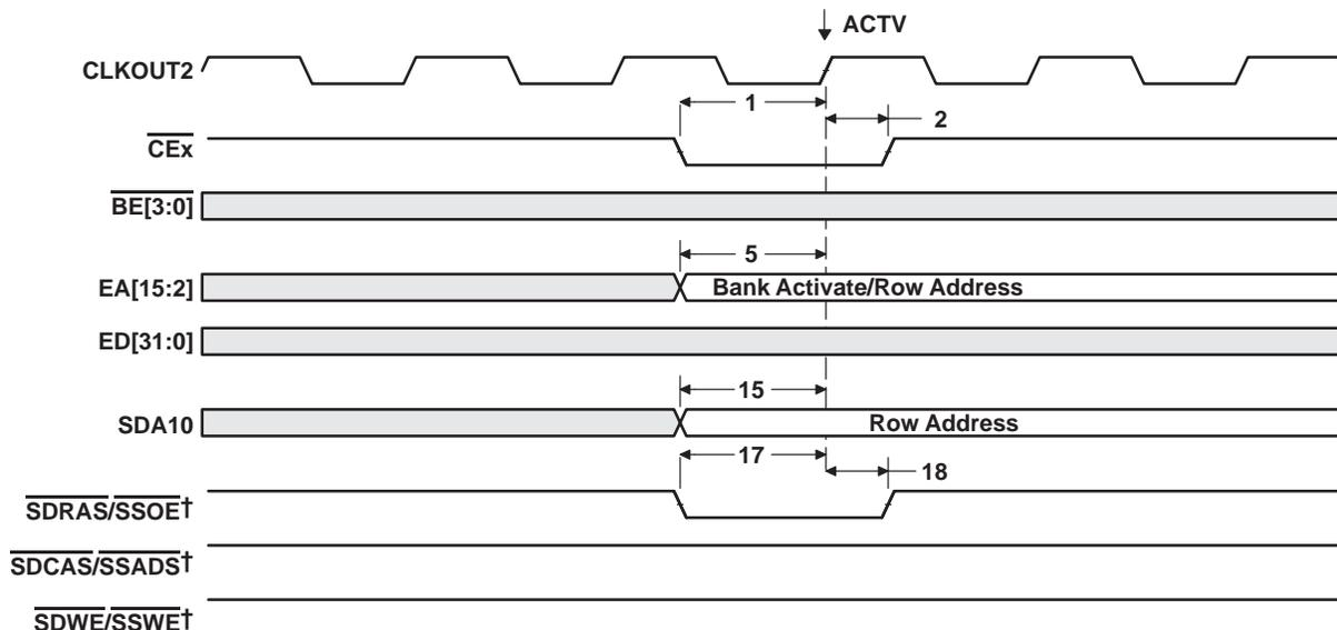
†  $\overline{\text{SDCAS/SSADS}}$ ,  $\overline{\text{SDRAS/SSOE}}$ , and  $\overline{\text{SDWE/SSWE}}$  operate as  $\overline{\text{SDCAS}}$ ,  $\overline{\text{SDRAS}}$ , and  $\overline{\text{SDWE}}$ , respectively, during SDRAM accesses.
