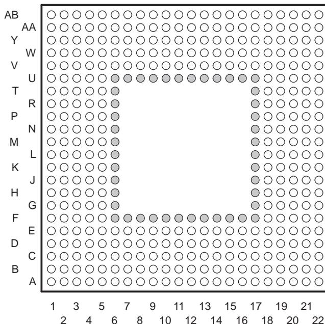
○ These balls are *NOT* applicable for the 'C6204 devices GLW 340-pin BGA package.
