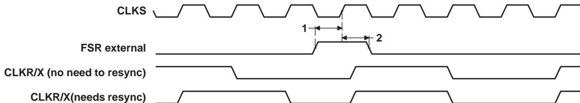
Figure 45. FSR Timing When GSYNC = 1
