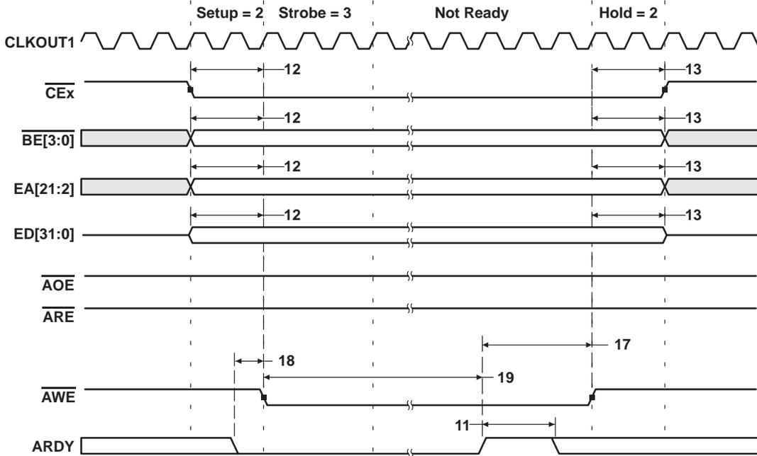
Figure 16. Asynchronous Memory Write Timing (ARDY Used)
