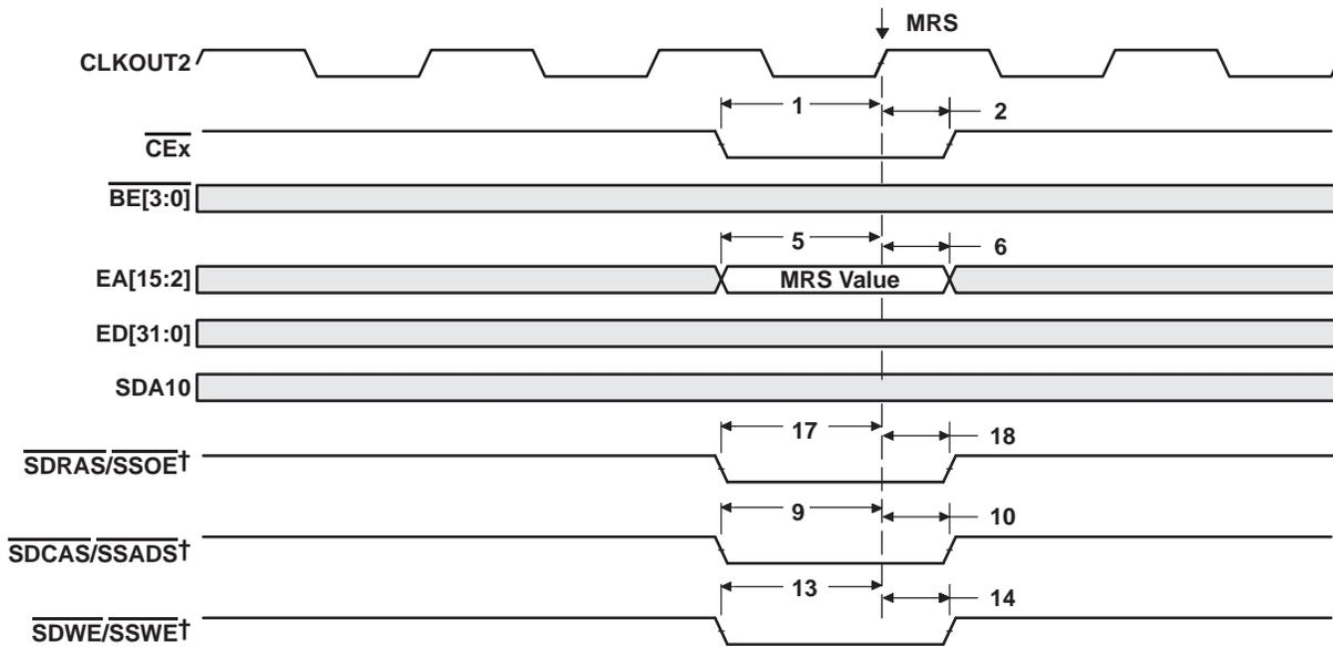
† SDCAS/SSADS, SDRAS/SSOE, and SDWE/SSWE operate as SDCAS, SDRAS, and SDWE, respectively, during SDRAM accesses.
