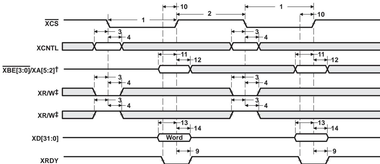
†  $\overline{XBE[3:0]}/XA[5:2]$  operates as byte enables  $\overline{XBE[3:0]}$  during host-port accesses.
