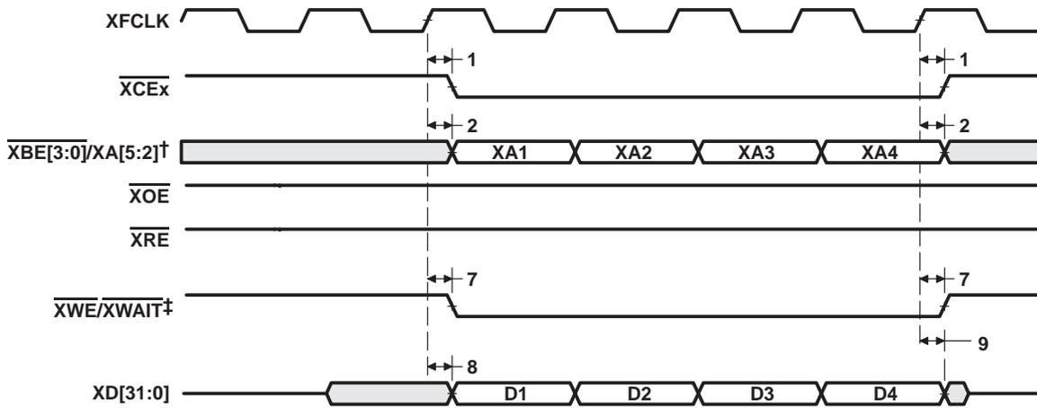
† XBE[3:0]/XA[5:2] operates as address signals XA[5:2] during synchronous FIFO accesses.
