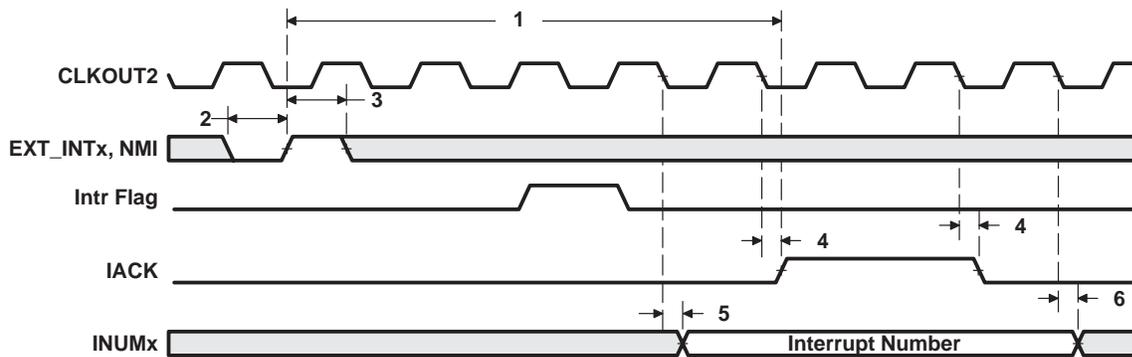
Figure 27. Interrupt Timing
