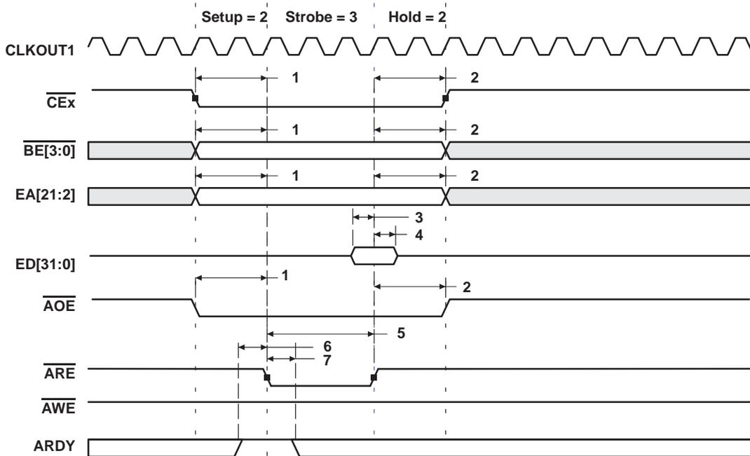
Figure 13. Asynchronous Memory Read Timing (ARDY Not Used)
