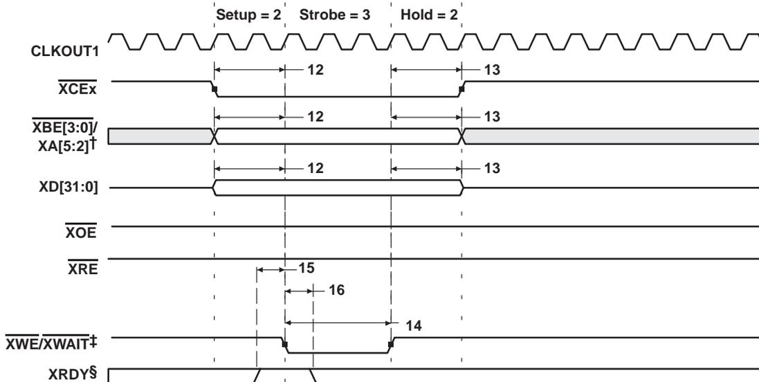
†  $\overline{XBE[3:0]}/XA[5:2]$  operates as address signals  $XA[5:2]$  during expansion bus asynchronous peripheral accesses.
