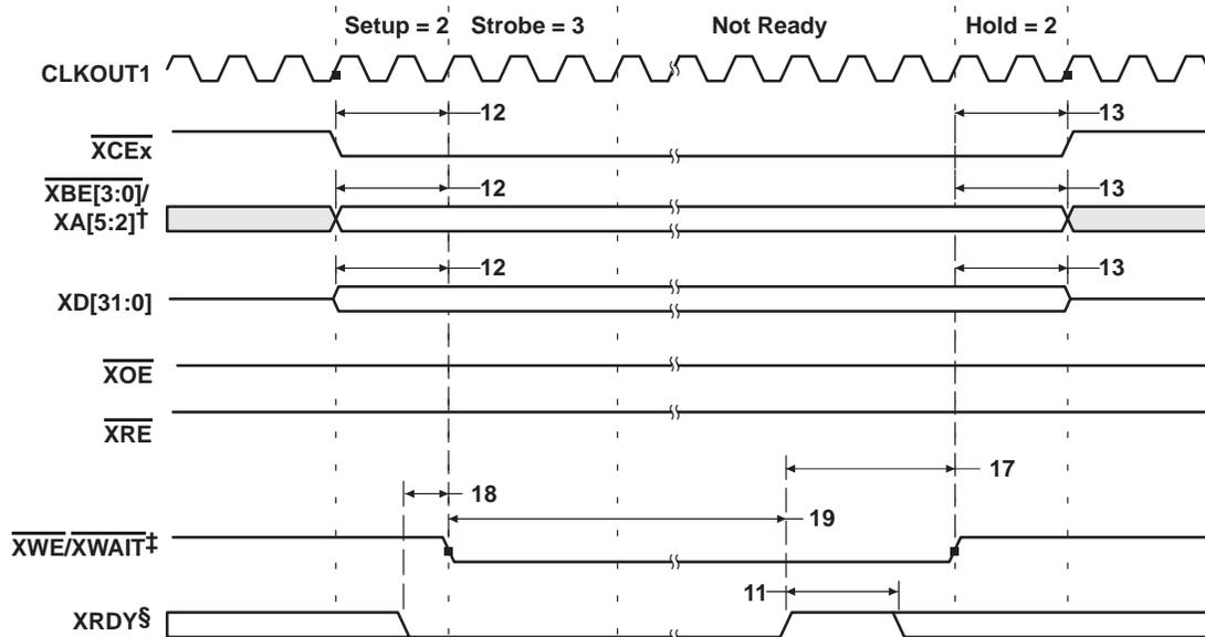
†  $\overline{XBE[3:0]}/XA[5:2]$  operates as address signals  $XA[5:2]$  during expansion bus asynchronous peripheral accesses.
