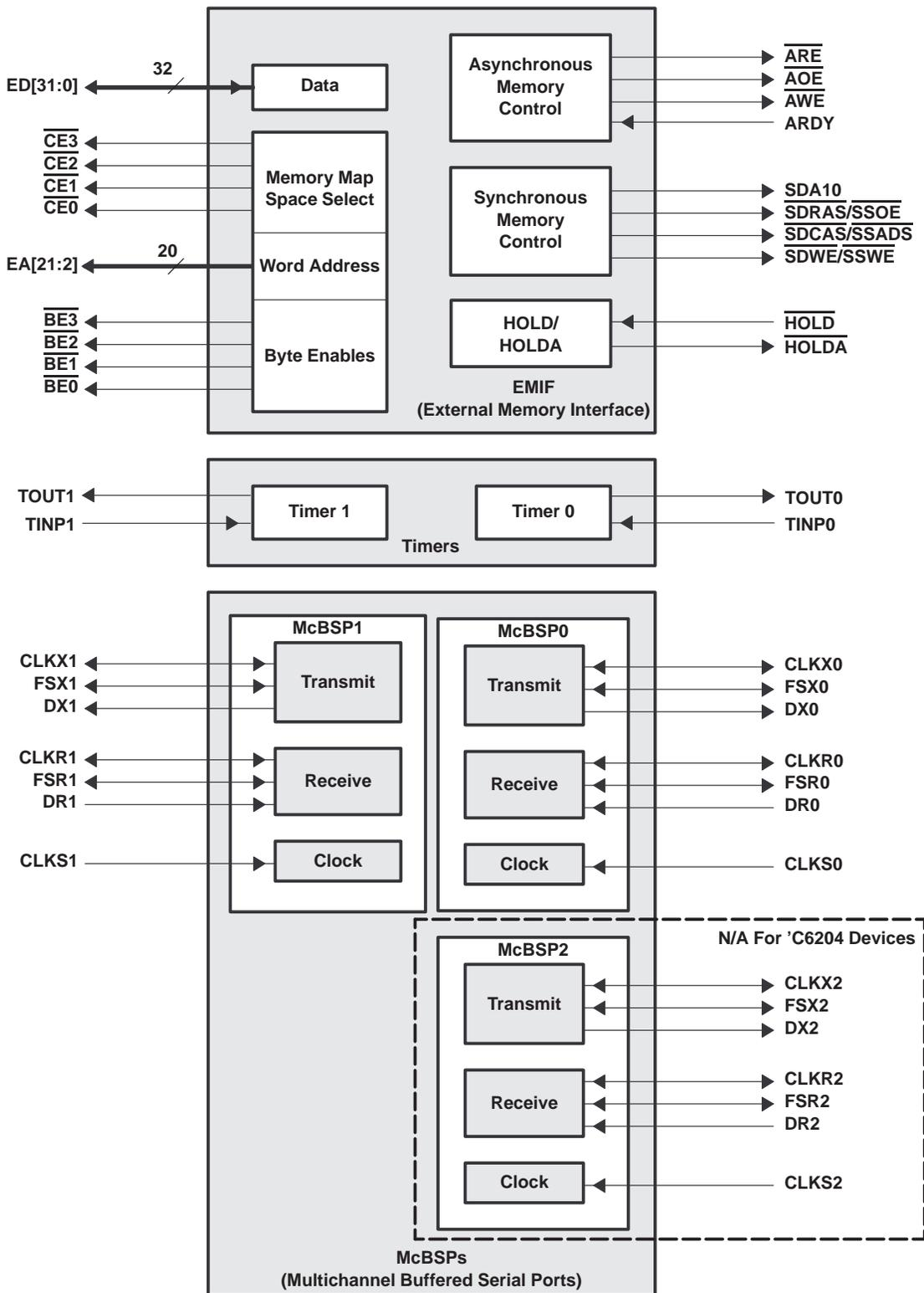
Figure 3. Peripheral Signals
