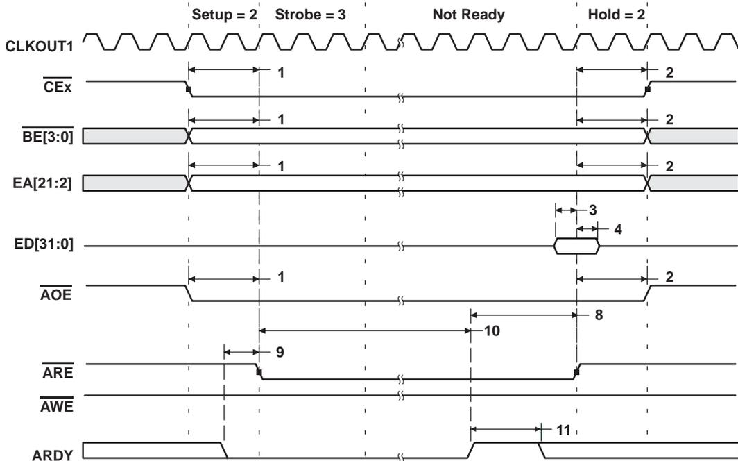
Figure 14. Asynchronous Memory Read Timing (ARDY Used)
