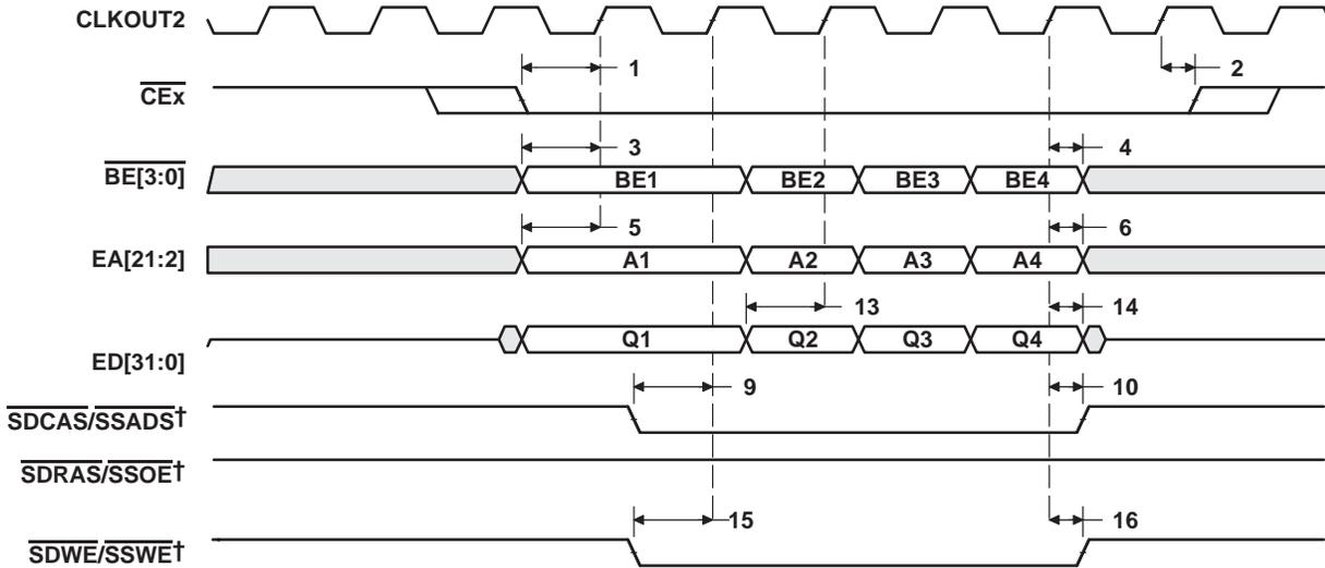
† SDCAS/SSADS, SDRAS/SSOE, and SDWE/SSWE operate as SSADS, SSOE, and SSWE, respectively, during SBSRAM accesses.
