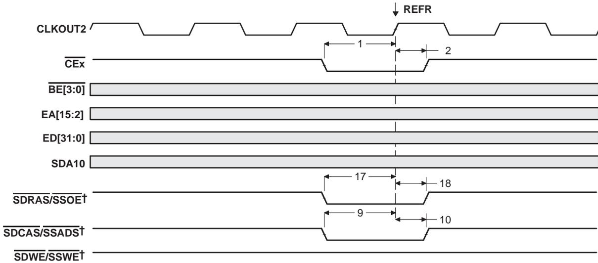
† SDCAS/SSADS, SDRAS/SSOE, and SDWE/SSWE operate as SDCAS, SDRAS, and SDWE, respectively, during SDRAM accesses.
