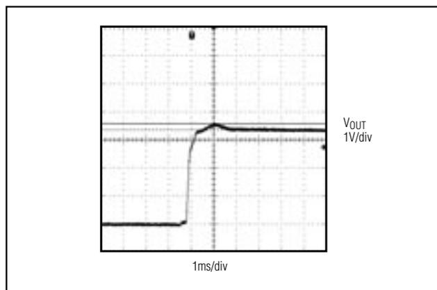
Figure 4. Turn-On Transient at Zero Load (4ms/div)
