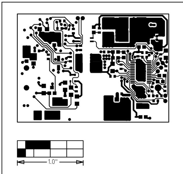
Figure 14. MAX5058 EV Kit PC Board Layout—Solder Side
