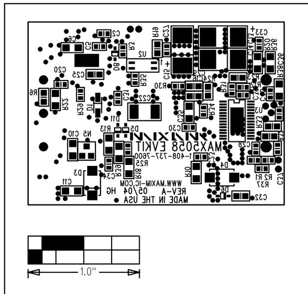
Figure 15. MAX5058 EV Kit Component Placement Guide—Solder Side
