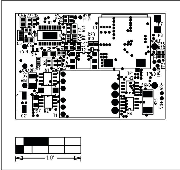
Figure 10. MAX5058 EV Kit Component Placement Guide—Component Side
