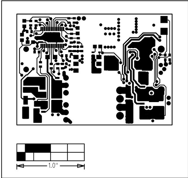
Figure 11. MAX5058 EV Kit PC Board Layout—Component Side
