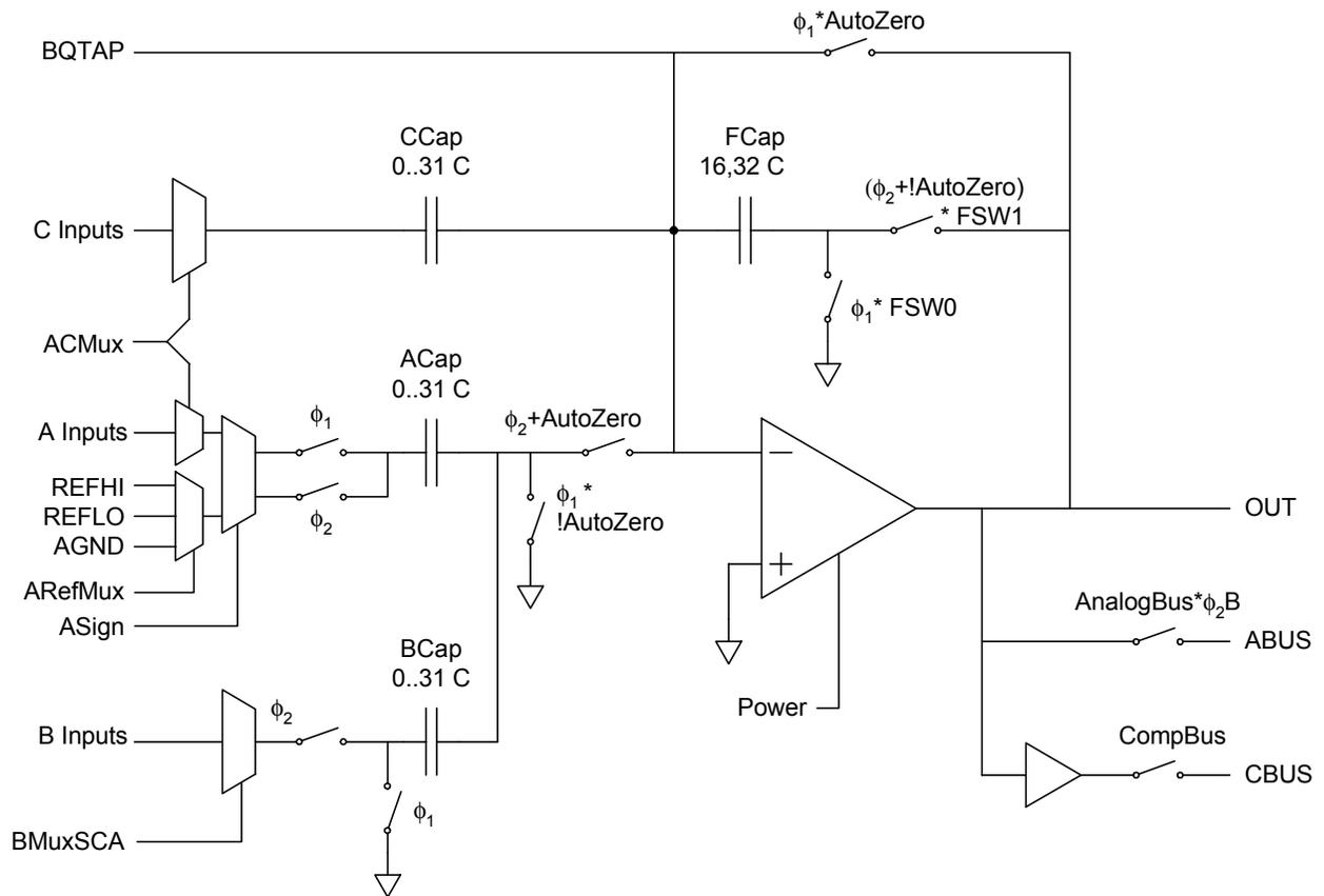
**Figure 21: Analog Switch Cap Type A PSoC Blocks**
