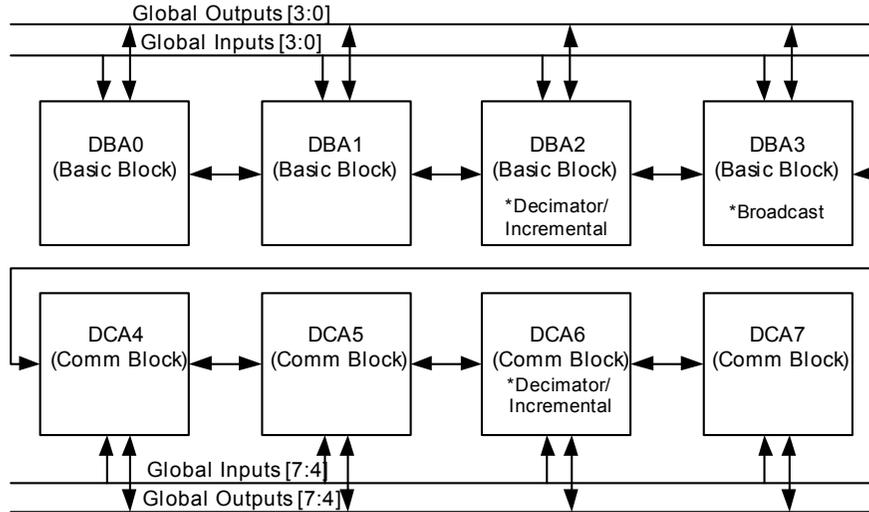
**Figure 12: Digital Basic and Digital Communications PSoC Blocks**
