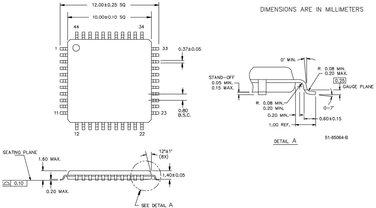
Figure 36: 44-Lead Thin Plastic Quad Flat Pack A44
