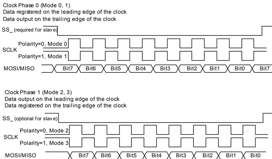
**Figure 15: SPI Waveforms**
