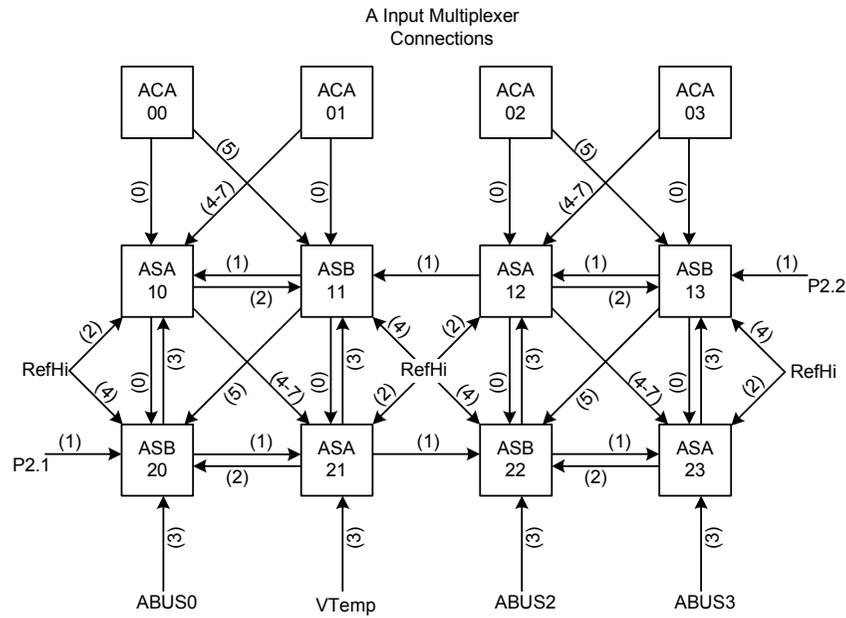
**Figure 22: AMux Connections**
