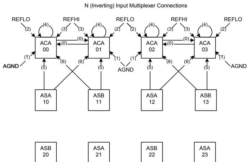
Figure 17: NMux Connections
