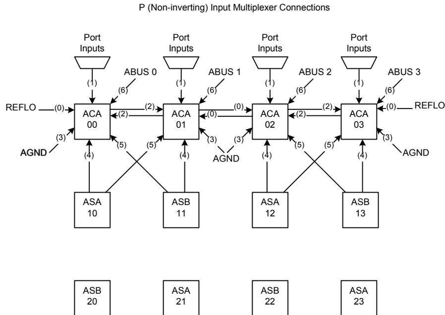
**Figure 18: PMux Connections**
