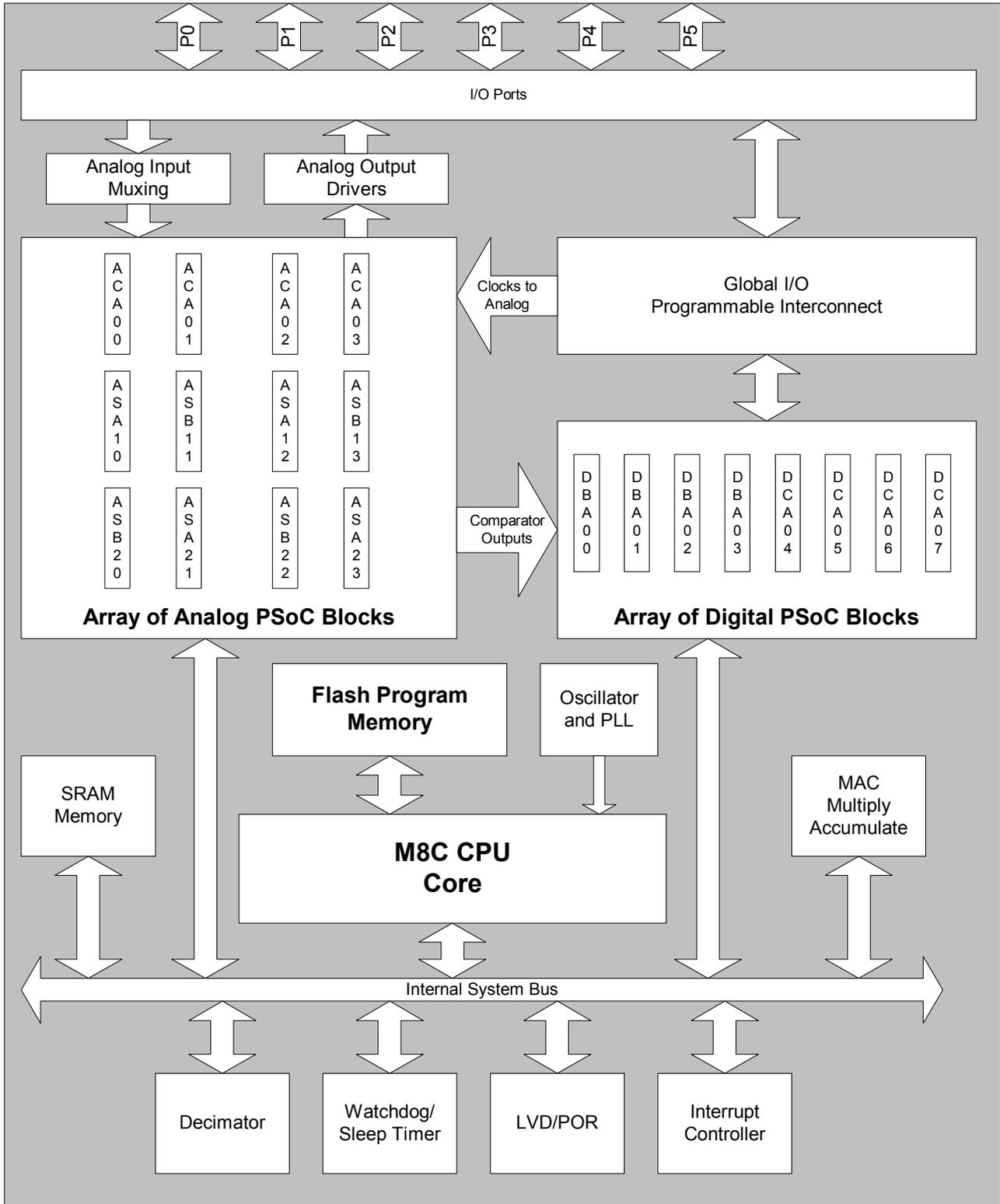
Figure 1: Block Diagram
