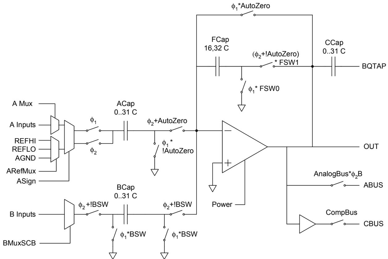
Figure 25: Analog Switch Cap Type B PSoC Blocks
