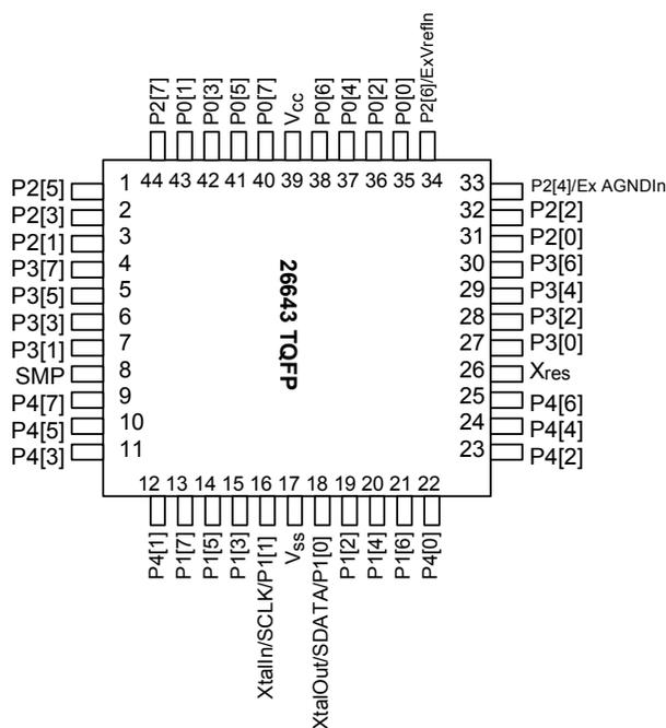
**Figure 5: 26643 TQFP**
