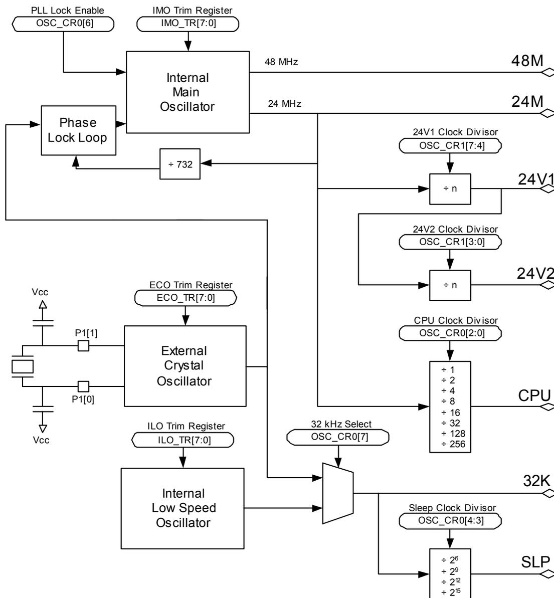
Figure 9: PSoC MCU Clock Tree of Signals
