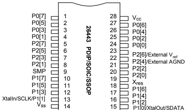
**Figure 4: 26443 PDIP/SOIC/SSOP****Table 5: Pin-out 44 Pin**
