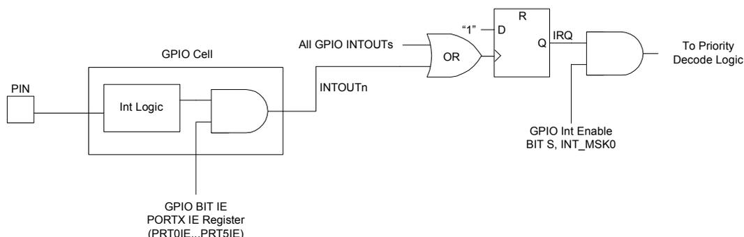
**Figure 11: GPIO Interrupt Enable Diagram**
