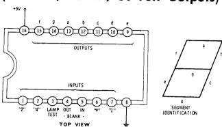
This package accepts a 1-2-4-8 positive-logic Binary Coded Decimal input and converts it to the proper pattern to light a 7-segment display. A low output is intended to light the segment.
