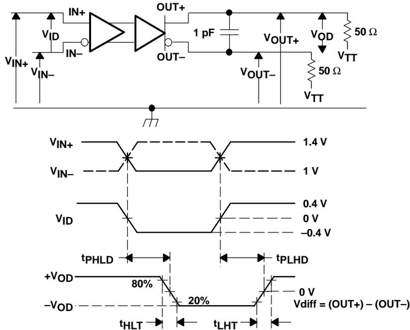
NOTE: All input pulses are supplied by a generator having the following characteristics:  $t_r$  or  $t_f \leq 0.25$  ns, pulse-repetition rate (PRR) = 0.5 Mpps, pulse width =  $500 \pm 10$  ns;  $C_L$  includes instrumentation and fixture capacitance within 0,06 mm of the D.U.T.
