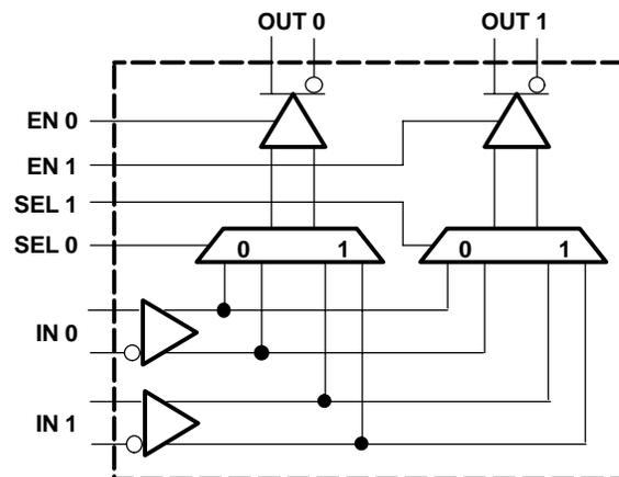
**EQUIVALENT INPUT AND OUTPUT SCHEMATIC DIAGRAMS**
