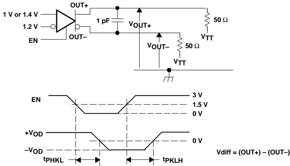
NOTE: All input pulses are supplied by a generator having the following characteristics:  $t_r$  or  $t_f \leq 1$  ns, pulse-repetition rate (PRR) = 0.5 Mpps, pulse width =  $500 \pm 10$  ns.  $C_L$  includes instrumentation and fixture capacitance within 0,06 mm of the D.U.T.
