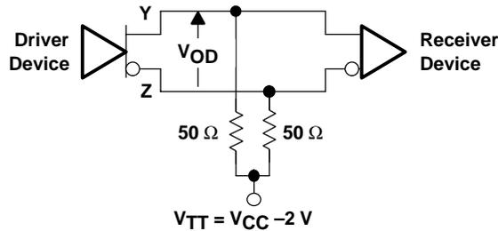
Figure 2. Typical Termination for LVPECL Output Driver
