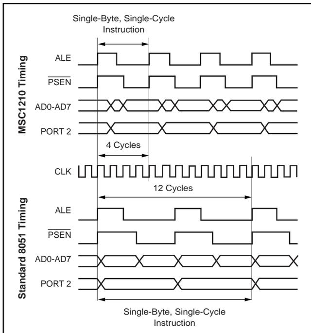
FIGURE 3. Comparison of MSC1211 Timing to Standard 8051 Timing.
