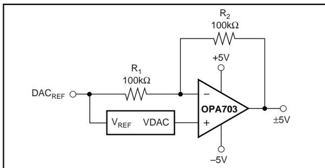
FIGURE 10. Bipolar Operation with the DAC.
