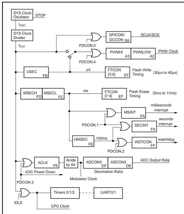
FIGURE 4. MSC1211 Timing Chain and Clock Control.
