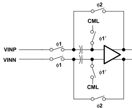
Figure 19. Analog Input Stage
