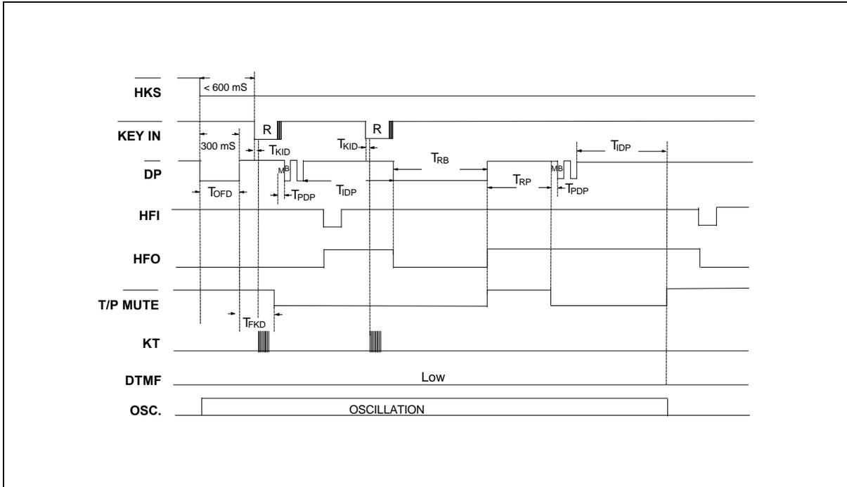
Figure 4. One-key Redial Timing Diagram (Pulse Mode)
