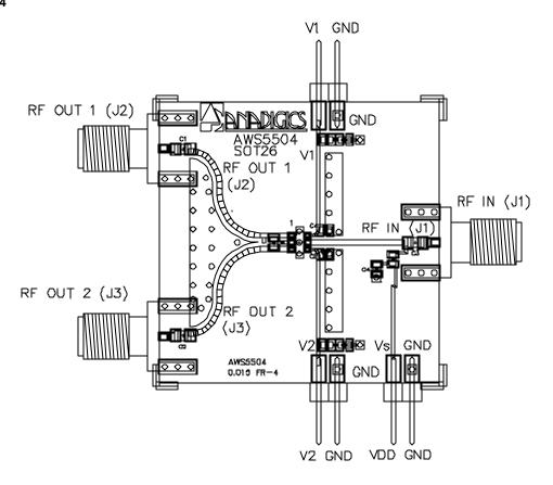
Figure 2: Test Circuit Schematic
